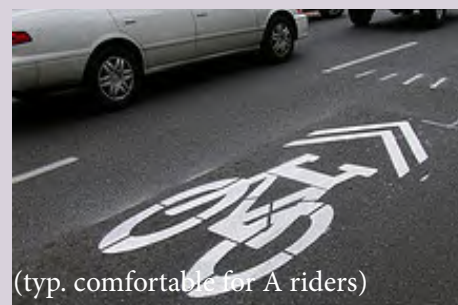
(typ. comfortable for A, B riders depending on speed and volume) bike lane: a separate lane for bicyclists
