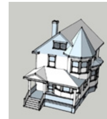
Left: The massing of the Foursquare with a 1-story porch reads as a cube with a shorter, more rectangular mass in front. Middle: The massing of the Queen Anne reads as a rectangle with a conical accent at the corner and a lower rectangle in front. Right: This end gable 2-story with a 1-story porch reads as a rectangular box perpendicular to the street with a shorter box in front.
