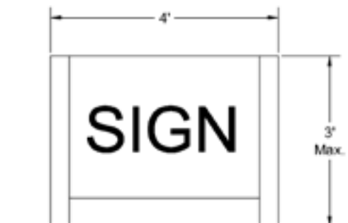
Left: How sign area is measured. Below: Appropriate handrails do not detract from the sloping front yards in the district.
